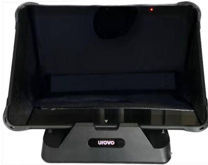
Figure 1- 9 Charge by desktop charger
